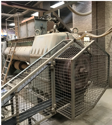
Clay moved into the extrusion machine
