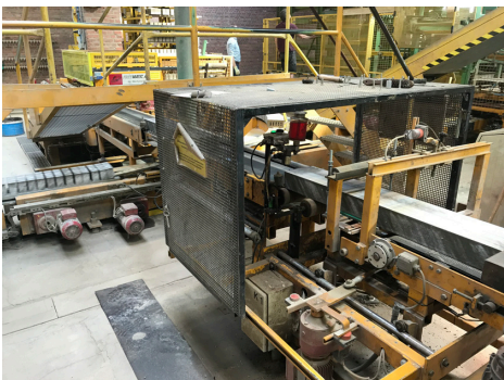
Compressed string of clay from which air was extracted in the vacuum environment
