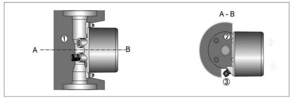
Figure 3-5: Heat insulation - cross-section
