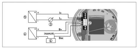
Figure 4-10: Electrical connection of pulse output
