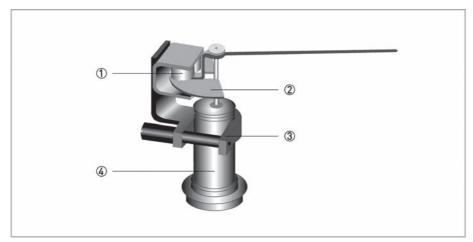
Figure 3-6: Pointer damping
