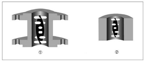
Figure 3-3: Types of magnetic filters
