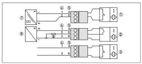
Figure 4-2: Connection terminals for limit switches
