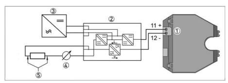
Figure 4-7: Power supply ESK4A with galvanic isolation
