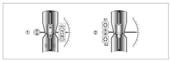
Figure 1-1: Measuring principle - general
