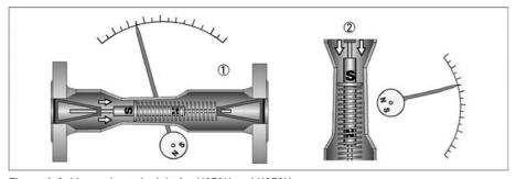
Figure 1-2: Measuring principle for H250H and H250U
