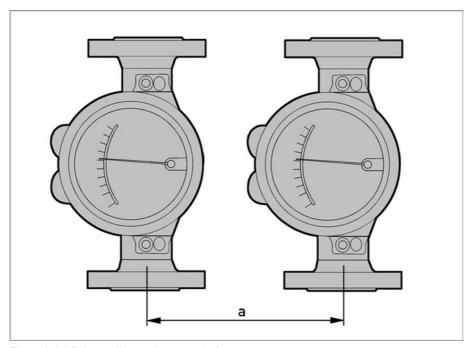
Figure 3-1: Minimum distance between devices
