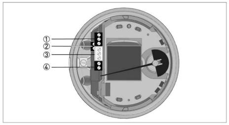
Figure 4-8: Position of the connection terminals
