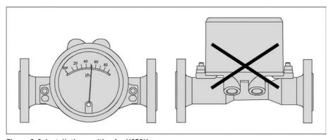
Figure 3-2: Installation position for H250H
