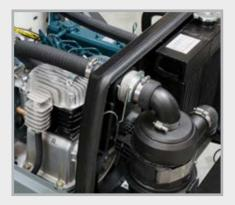
The extremely powerful 4-cylinder engine is exceptionally quiet due to the speed of only 2,600 rpm and extremely effective sound insulation.
