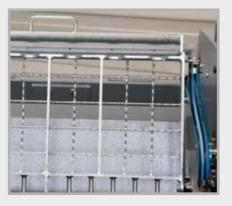
The intelligently positioned water metering pipe prevents blockages and the optional patented dust extraction system ensures a convenient filling process.
