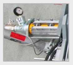
The powerful 2L6 worm pump with M 50 pressure connection is included as part of standard equipment. It can process site-made mixes with up to 6 mm grain size, depending on the desired delivery rate and the properties of the material.
