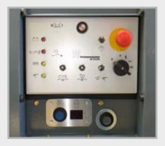
The clearly laid out operating panel enables users to control the machine easily and in accordance with CE standards. The delivery rate and water metering are infinitely variable.
