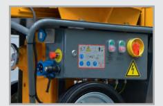
Central control cabinet is also a power distributor for attached devices such as a pan mixer or compressors
