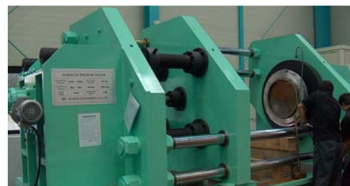
Hydrostatic Shell & Seat Leakage Tester
