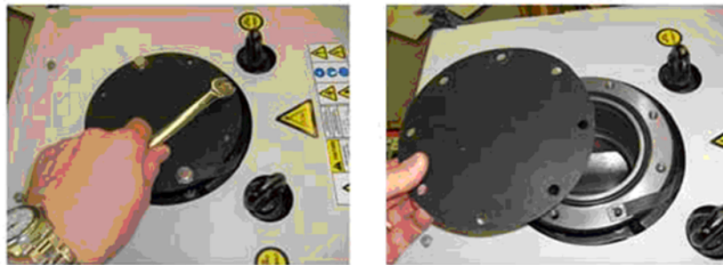
Figure 5 - Connecting the pump inlet
