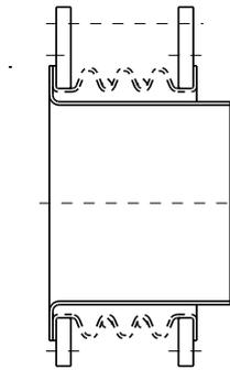
Fig. 4 FLUROFLEX® "FXS internal smoothbore sleeve"
