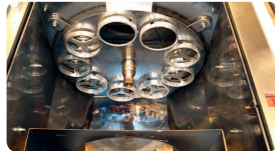
Double rotating wafer holder with 9 pcs. 4" wafer holders
