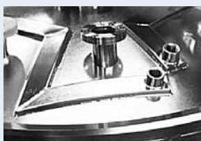
Water channel construction
