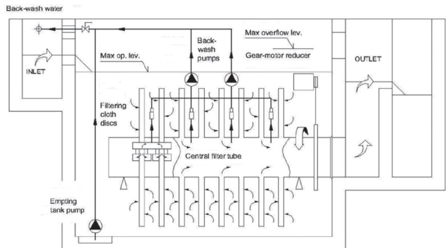
Typical flow diagram of MITA disc filter
