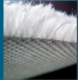
The material coating the filter drums and discs is of the “pile” or “free-fibre” type.
