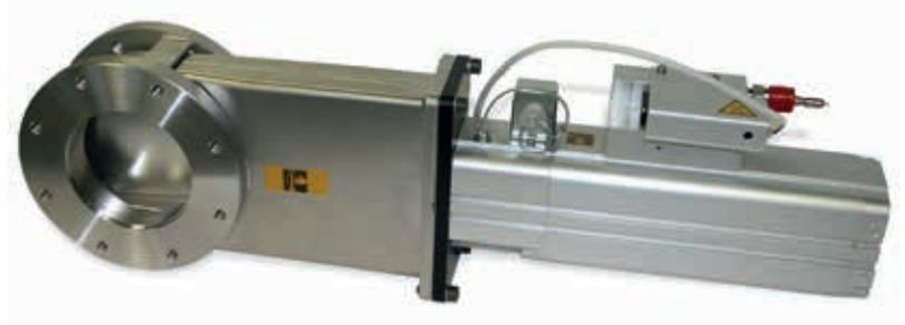
The unique Lock-Out-Tag-Out (LOTO) safety mechanism allows personnel to freely work on the vacuum system without fear of the valve inadvertently opening. The valve is physically held closed using a pin to lock the valve shut preventing it from being opened. If there is a requirement for the valve to be locked shut, a lockout hasp can be inserted through the LOTO pin and padlocked.
