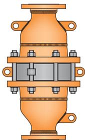
The combination of our unique patent pending High Energy Dissipation System (HEDS™) design and E-Flow™ technology elements attenuate the shock wave and extinguish the flame mitigating the effects of an explosion by preventing its propagation. The UCA Series detonation arrester uses an optimised crimped ribbon element which allows gas or vapour to pass with minimal pressure loss. Designed to withstand the worst case scenario of unstable detonation, the
