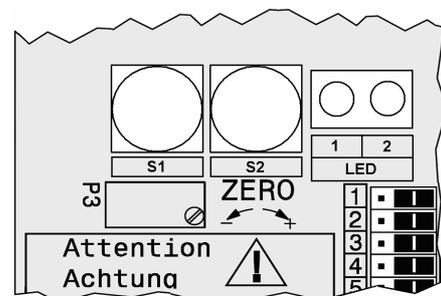
**Adjusting the end of the measuring range (20mA)**
