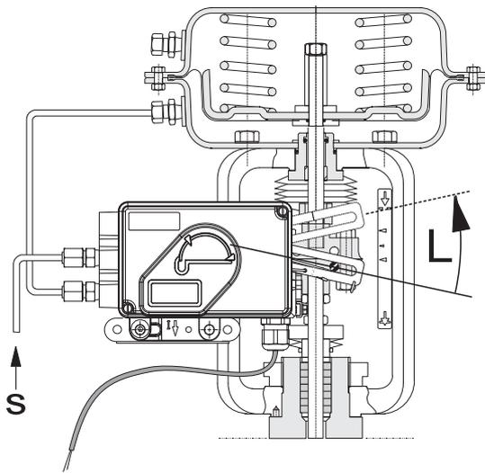
Defined as direction of rotation of feedback shaft from the start to the end position, looking at the positioner from the front. Switch 1+2 to "R" if necessary.
