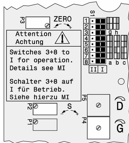
**5 Setting and Start Up of position transmitter 4-20mA**
