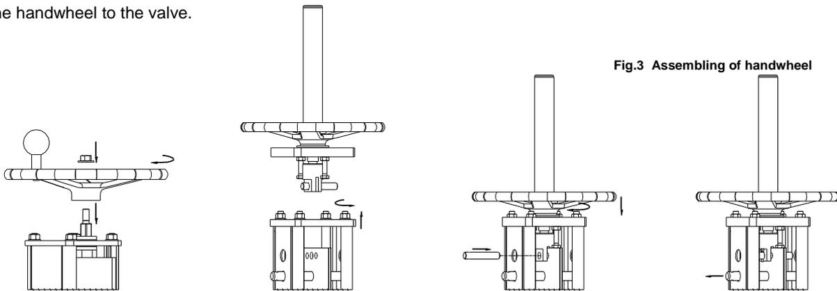
Fig.3 Assembling of handwheel
