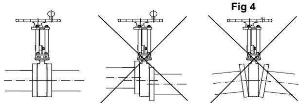
If the flanges and the valve are not centred, the valve may be damaged by erosion and a dirt pocket may occur which can lead to clogging and corrosion of the valve.
