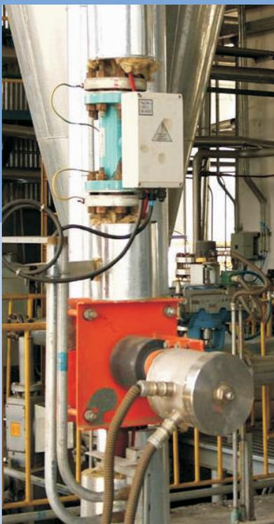
Installation on a pneumatic conveying line, with a *DYNAvel* velocity sensor.
