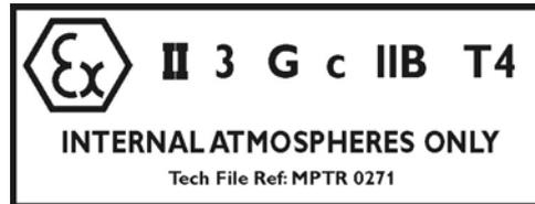
This equipment is designed to meet the requirements of Group II Category 3 equipment in accordance with Directive 94/9/EC of the European Parliament and the Council of 23rd March 1994 on the approximation of the laws of the Member States concerning equipment and protective systems intended for use in potentially explosive atmospheres. (The ATEX Directive).
